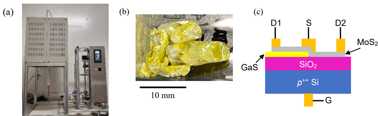
Figure 1 (a) Single-crystal growth system by the Bridgman method. (b) GaS single crystals grown by the Bridgeman method. (c) Schematic diagram of a MoS 2 field-effect transistor with GaS as a buffer layer.
